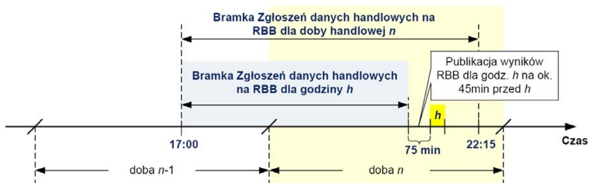
Figure 10: The schedule of the intraday market suggested in the new Polish electricity market design (source: PSE-Operator S.A.)
