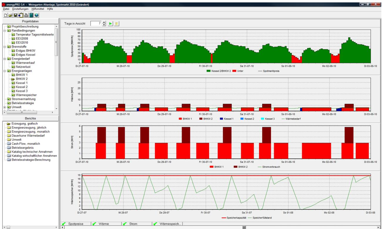
**Figure 2: Simulated operation in the Spot Market of Badenova WÄRMEPLUS's 6 MW-Combined Heat and Power-plant in Freiburg-Weingarten.**
